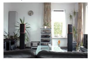
look that is so subtle, it nearly disappears. One Tower in each corner of the room produces bass mode control down through 40 Hz and treble range diffusion which backscatter at 400 Hz and above. This high efficiency corner bass trap delivers the same high power acoustic punch as provided by all ASC TubeTrap products.
